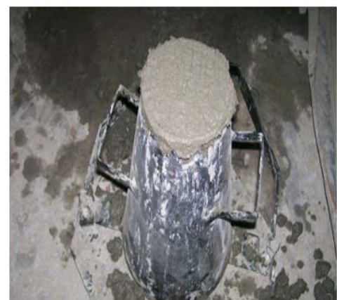
FIG.6 slump test before lifting
